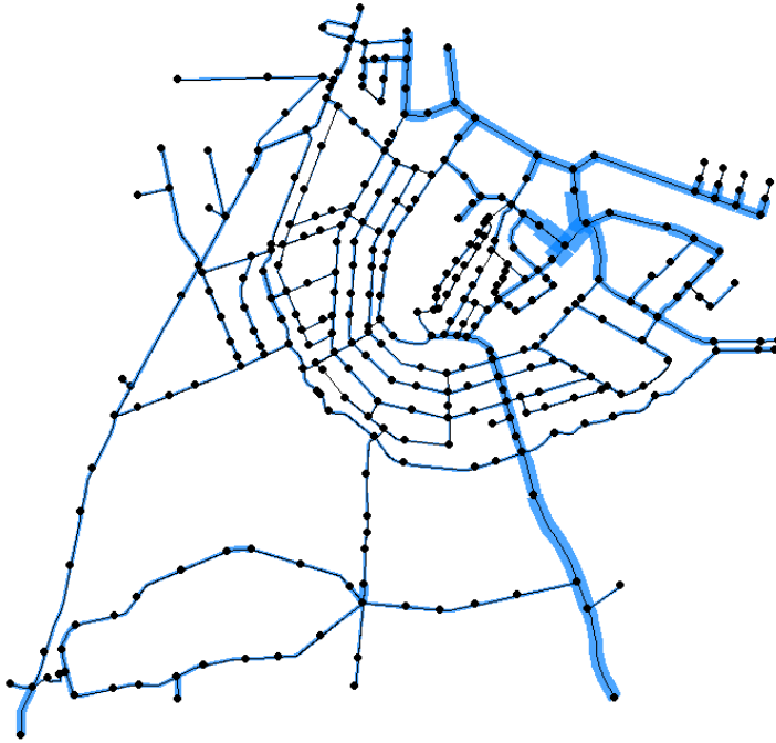
Figure 3: The network definition. Line width proportional to the width of the canals.
